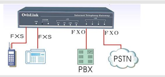
**FXO:** The FXO ports connect to the PSTN line (analogue telephone line) or company's PBX line (the line to the extension phone). It allows the VoIP device to communicate with the ordinary telephone system. Having the PXO port is necessary if you want your device to link with PBX or outside telephone line.
